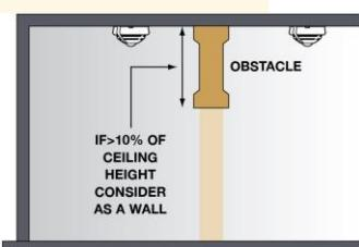
Applies to floor and ceiling void. Any of the above detector positions are acceptable.
