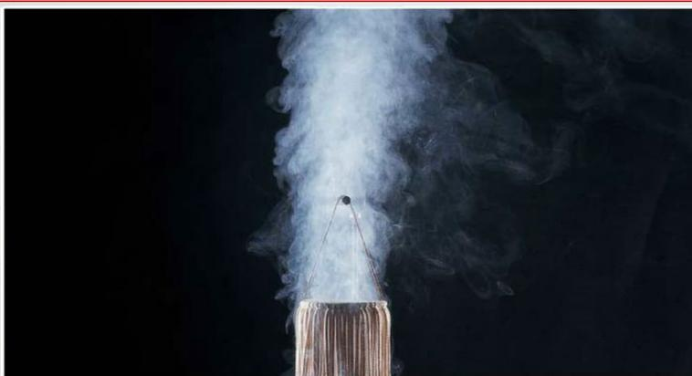
Test fire 3: glowing smoldering fire (cotton)
