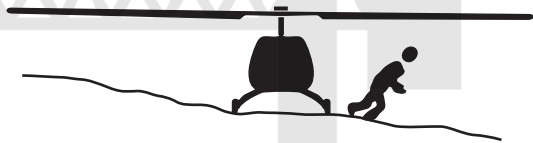
Fig. 12-4.4.16-2 Personnel Approach/Departure Path (Sloping Ground)
