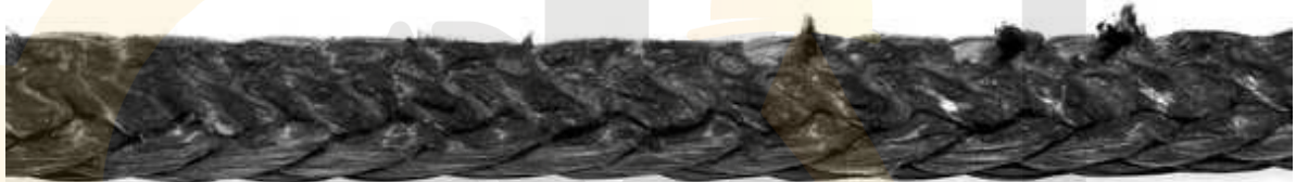
Figure 30-2.8.2-5 Melt Damage Due to Heat
