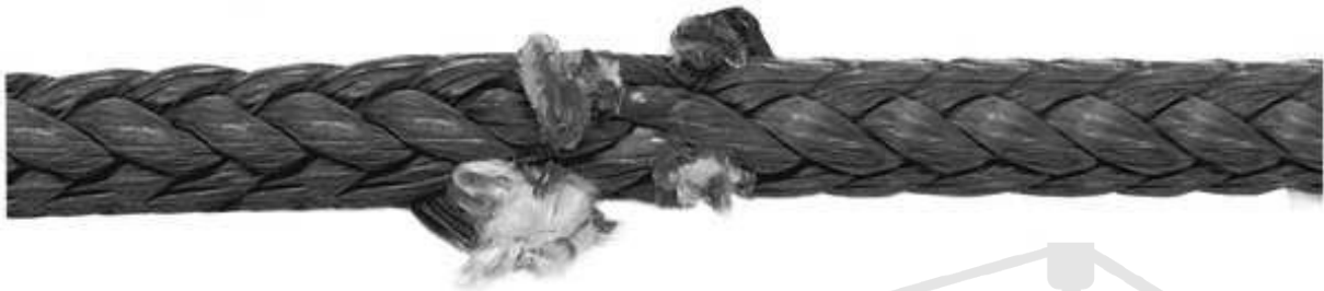
Figure 30-2.8.2-1 Cuts, Gouges, and Yarn Material Breakage
