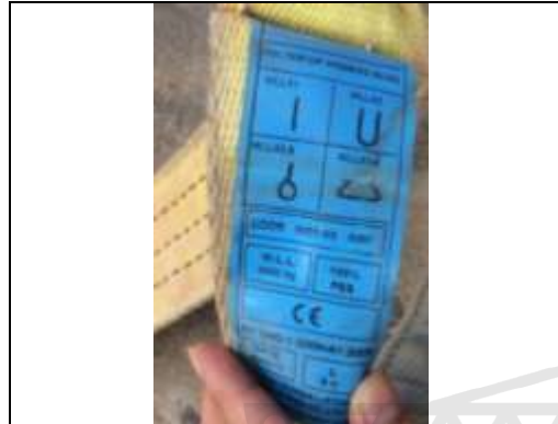
Example of tag on polyester webbing sling showing the WLL factors
