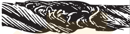
Rope that has been jammed after jumping off sheave
