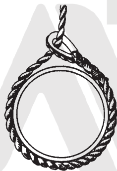
Correct – Use thimbles in the eyes.
