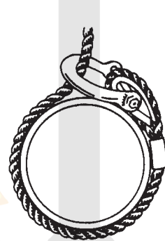
Correct – Shackle pin cannot turn.
