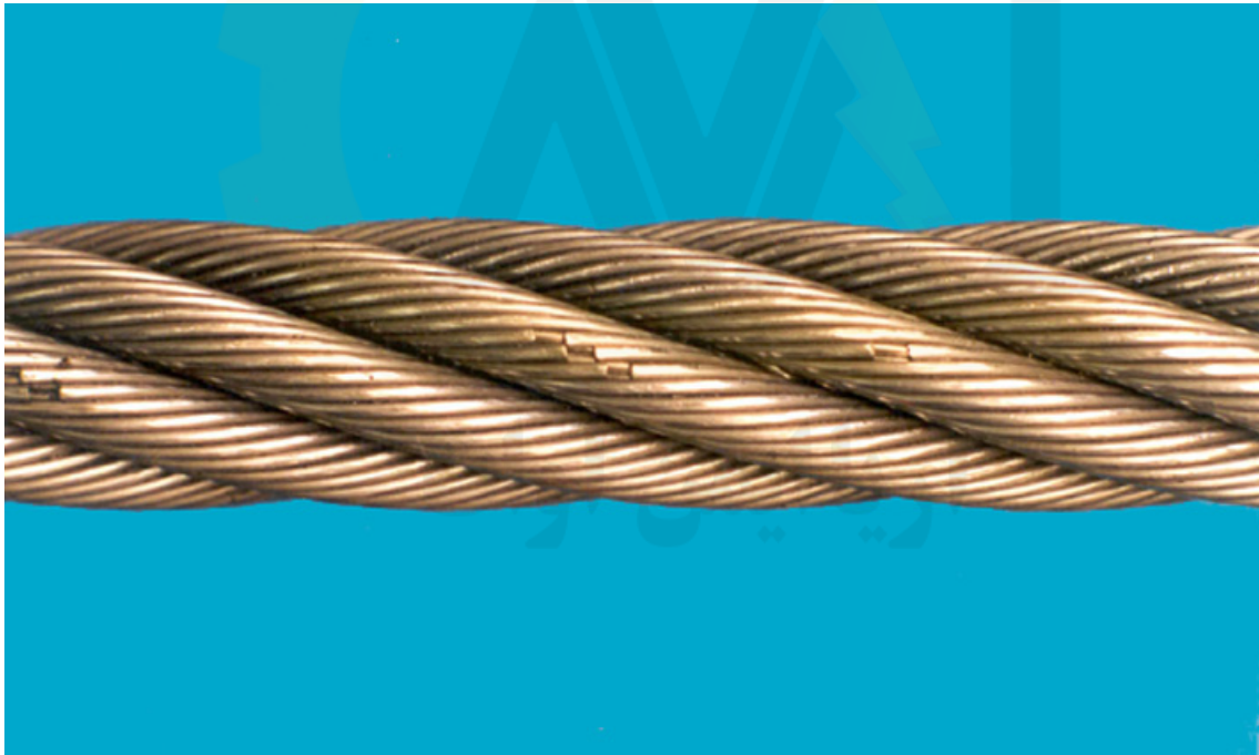
Figure B.13 — Crown wire breaks
