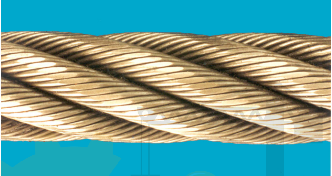
Figure B.10 — External wear
