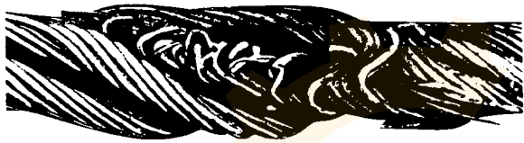
A rope that has been jammed after jumping off a sheave.
