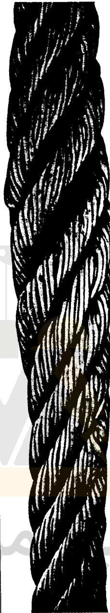
Localized Crushing of Rope
