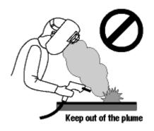
Natural dilution ventilation should not be used to ventilate confined spaces, an area that has a structural impediment to natural airflow, or when the airborne contaminant contains a carcinogenic substance, or other substance of high toxicity. See CSA W117.2 for specific guidance.
