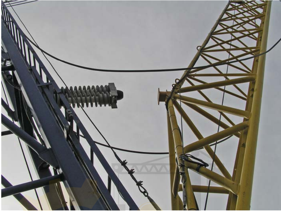
Figure 17a – Longer Springs in the Spring Buffer and Jib “make up piece”
