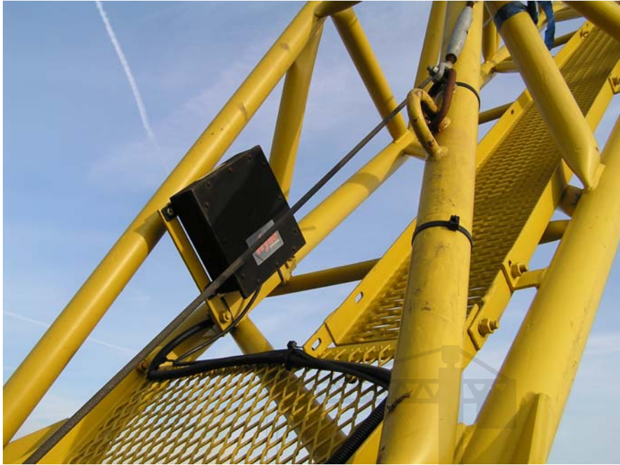
Figure 12a – Crane Inclinometer fitted close to the pivot end of Jib Section 1
