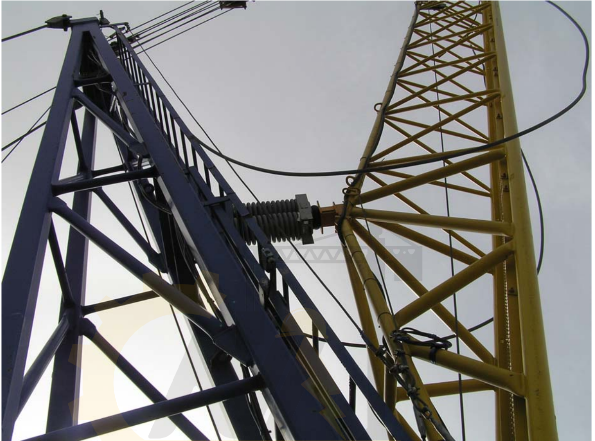
Figure 17c –Compression of the longer springs in the Spring Buffer at a jib angle of nominally 86°
