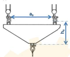
The selection of the spreader or equalizer beam has to be done carefully and along with the dimensioning of the beam (Safe Working Load), the geometry has to be taken into account. The effect described in Annex 1 can also happen when using equalizer beams.
